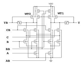
Fig. 5. Schematic diagram of pseudo-dynamic element XOR3M
