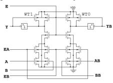
Fig. 4. Schematic diagram of pseudo-dynamic multiplexer 2:1
