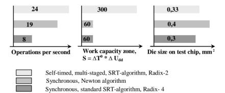
Fig.7. Results of different variants of computing device implementation testing
