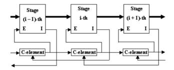
Fig. 1. Arrangement of request-acknowledge interaction between stages of computing device
